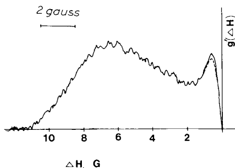
Fig. 2. NMR half-derivative curves for a blend containing 2 wt % EVA in PVC: (---) milled sample; (—) blend heat treated 20 min at 170°C.
